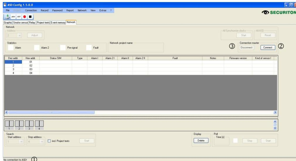
The "Connect" button ② is used to establish the connection between the PC and the SMM 535 Master Module (and therefore the network). The message bar now reads: "Connected with the Master Module!". The "Disconnect" button ③ can be used to clear down the connection with the SMM 535 Master Module.
