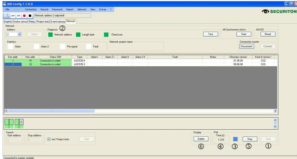
The green flashing diagnostics displays ② and the blue flashing visualisation display ③ signal the active communications within the network. The poll time [s] ④ also indicates the instantaneous latency (network response time) in seconds. The "Stop" button ⑤ is used to stop the visualisation. The "Delete" button ⑥ is used to delete the entire current network display in order to carry out a new network search.
