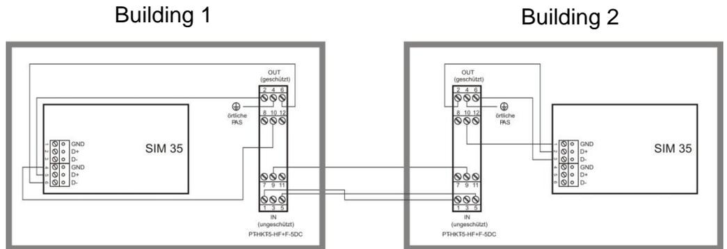
Connection for a network with repeaters (with repeaters on either side at the building transfer point)
