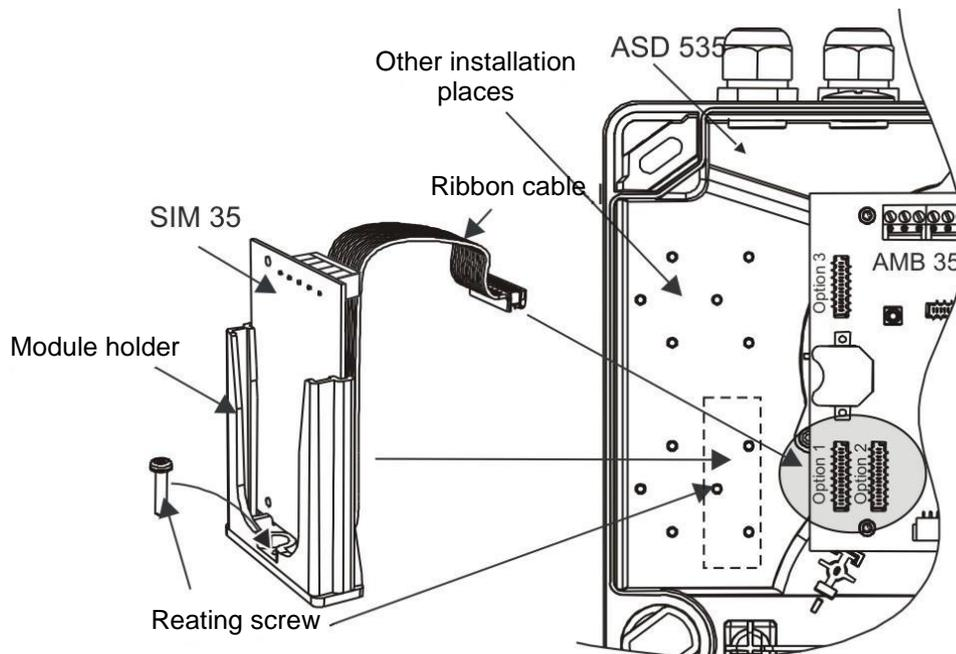
When retrofitting the SIM 35 to existing ASD 535 detectors, de-energise the ASD 535 first, then mount the SIM 35, then reconnect the ASD 535. Once the ASD 535 is energised, the SIM 35 is automatically detected and is, from that moment onwards, monitored by the ASD 535. Fitting the SIM 35 has no influence whatsoever on the existing configuration of the ASD 535.
