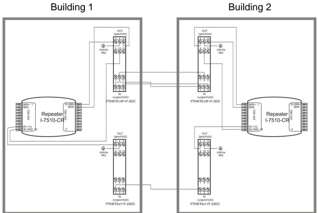
The overvoltage protection modules have a standard top-hat rail connection and are fitted into a corresponding top-hat rail housing (e.g. GEH EXB set) or a top-hat rail cabinet (e.g. B6-CTR-2).
