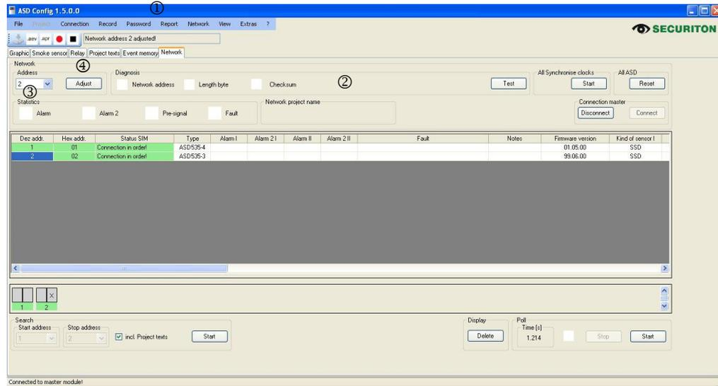
All the configurations that are available with a local connection to an ASD 535 can also be made via the network. The only exception is carrying out an initial reset and uploading new firmware. The two settings are made exclusively using a local connection to the ASD 535.
