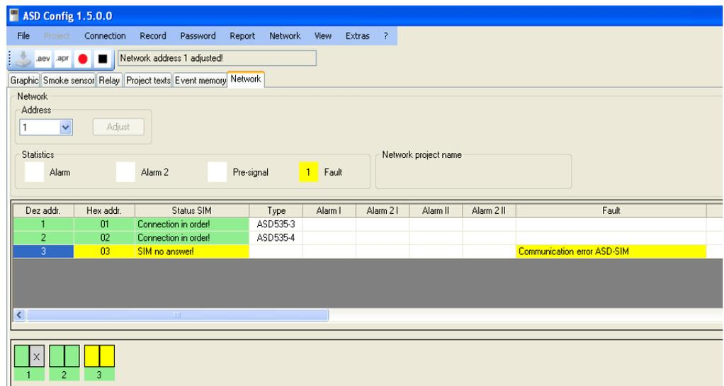
Indication of a front panel fault
