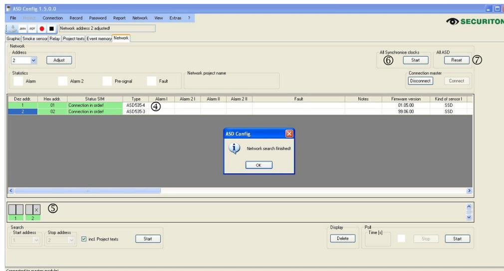
A green display indicates that the network participants are ready (SIM status column "Connection in order"). The icon view ⑤ displays two rectangles for each ASD 535; they symbolise the fitted smoke sensors. An X inside a rectangle indicates that the smoke sensor is not fitted (e.g. with ASD 535-1 or ASD 535-3). The "Start" button ⑥ is used to synchronise the clocks of all the ASD 535s with the PC's system time; the "Reset" button ⑦ is used to reset all the ASD 535s in the network.
